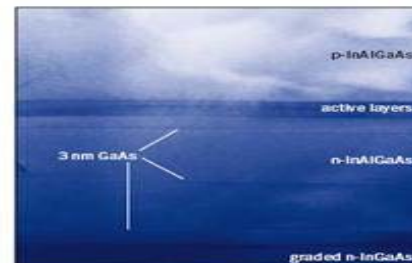
Annealing removes the dislocations in InGaAs epilayers with a metamorphic buffer, according to transmission electron microscopy studies.
